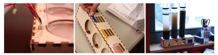
Figure 2. Designing a bio-electronic system: column plugged into casing; labeling the column slots; testing the system.
